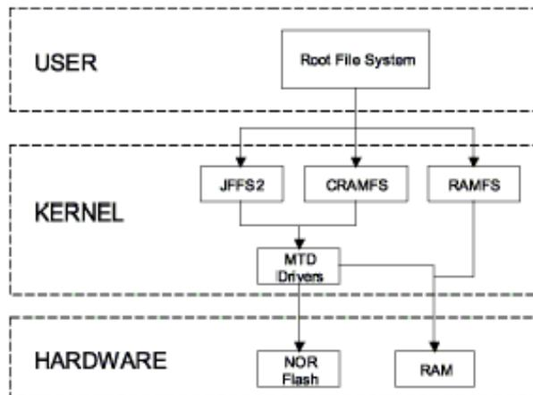
**Figure 28-1. Components of a Flash-Based File System**
