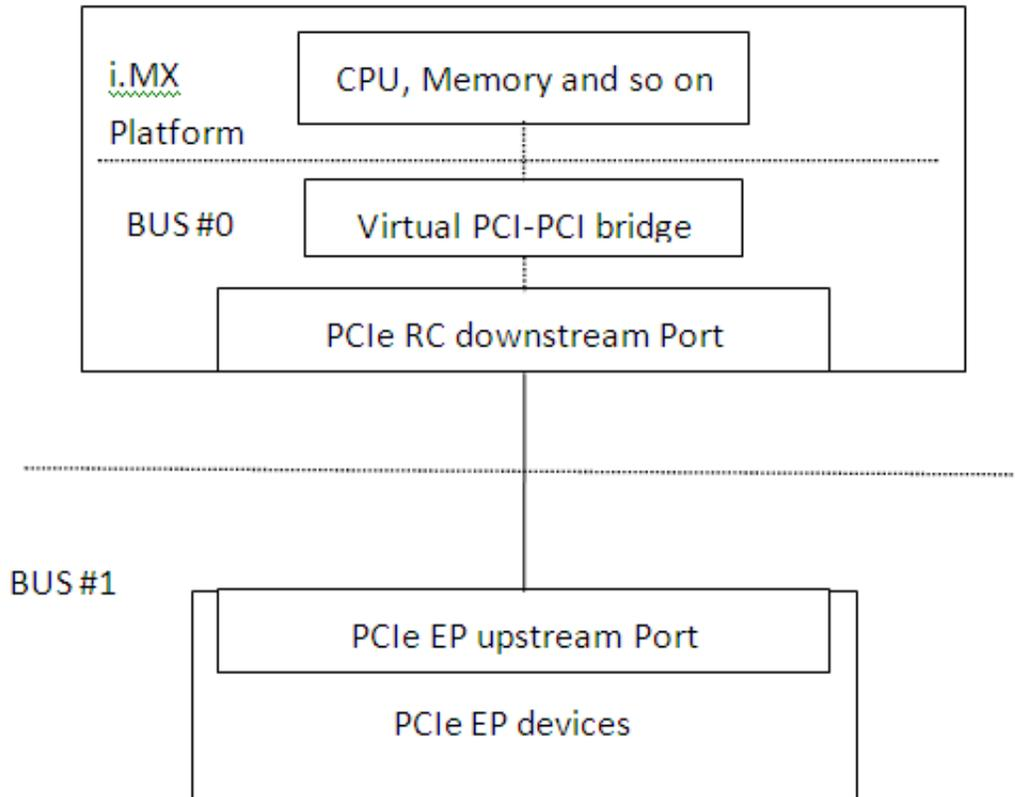
**Figure 36-1. diagram of the PCIe RC port on i.MX 6**
