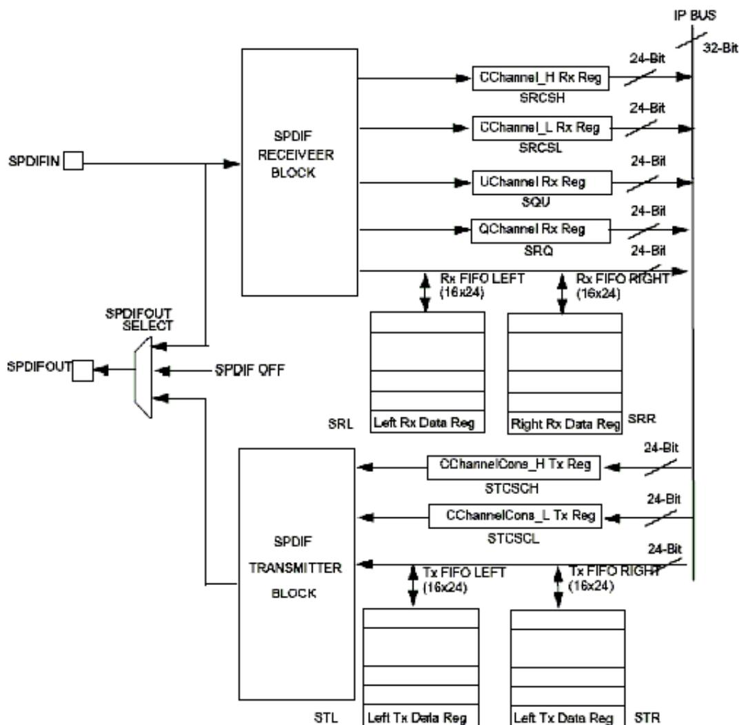
Figure 27-1. S/PDIF Transceiver Data Interface Block Diagram
