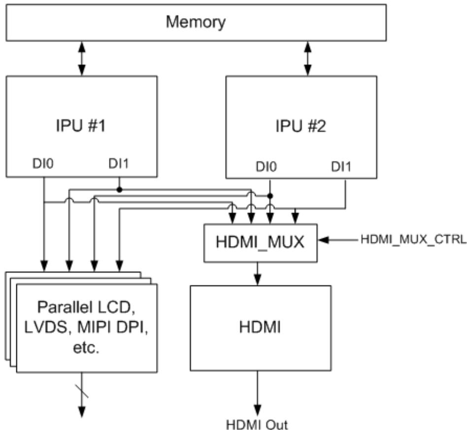
**Figure 13-2. IPU-HDMI Hardware Interconnection**
