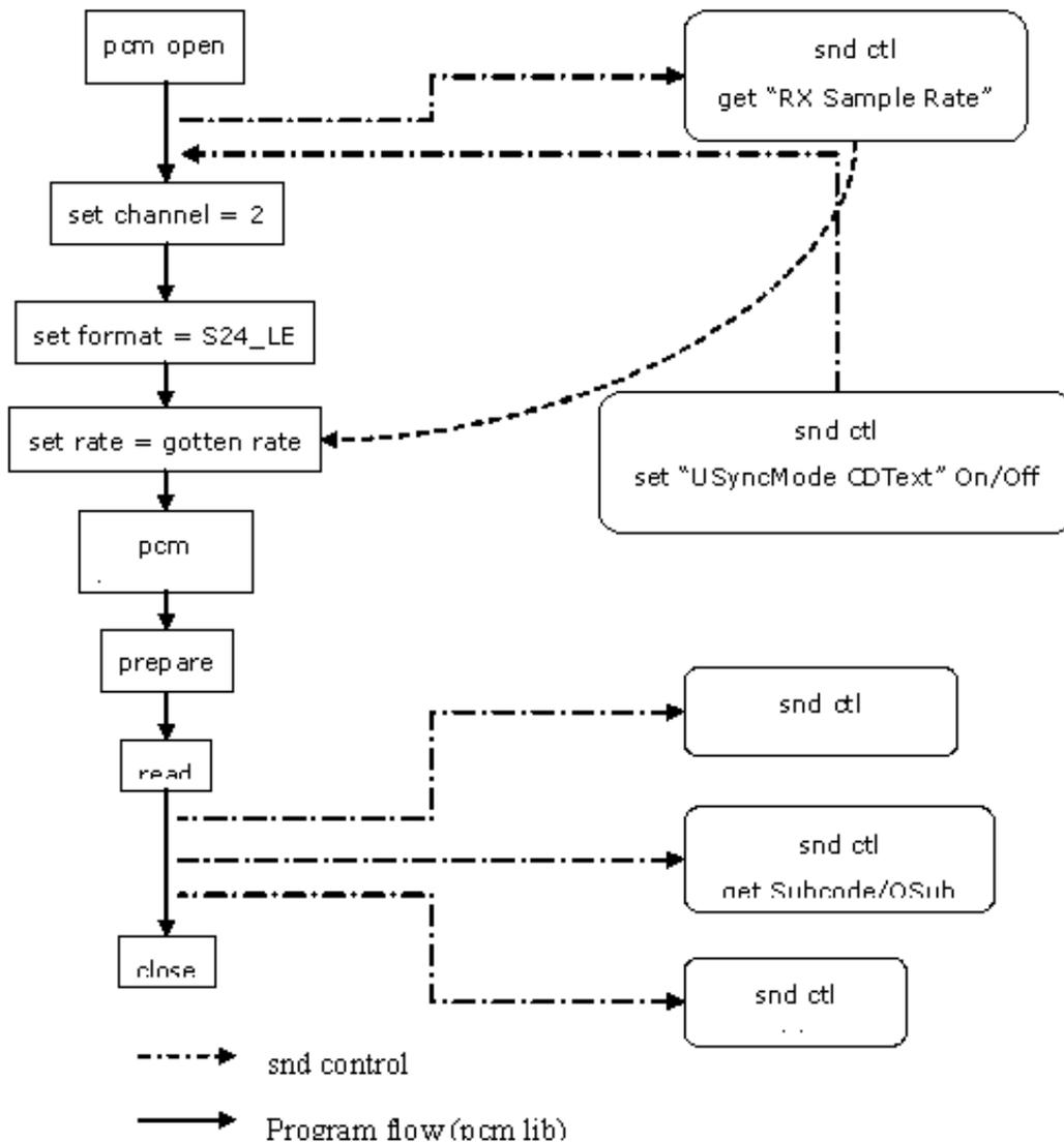
Figure 27-2. S/PDIF Rx Application Program Flow
