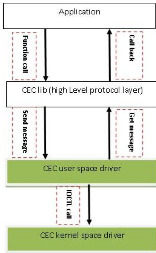
Figure 13-4. HDMI CEC SW Architecture
