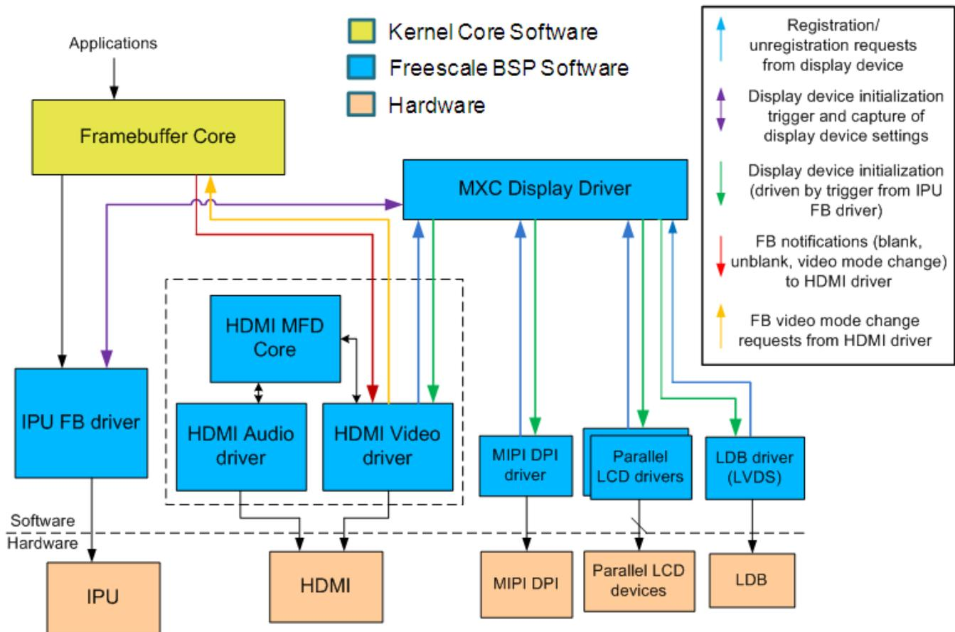
Figure 13-3. HDMI Video SW Architecture
