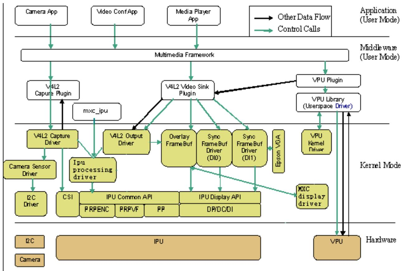
**Figure 6-2. Graphics/Video Drivers Software Interaction for IPUv3**
