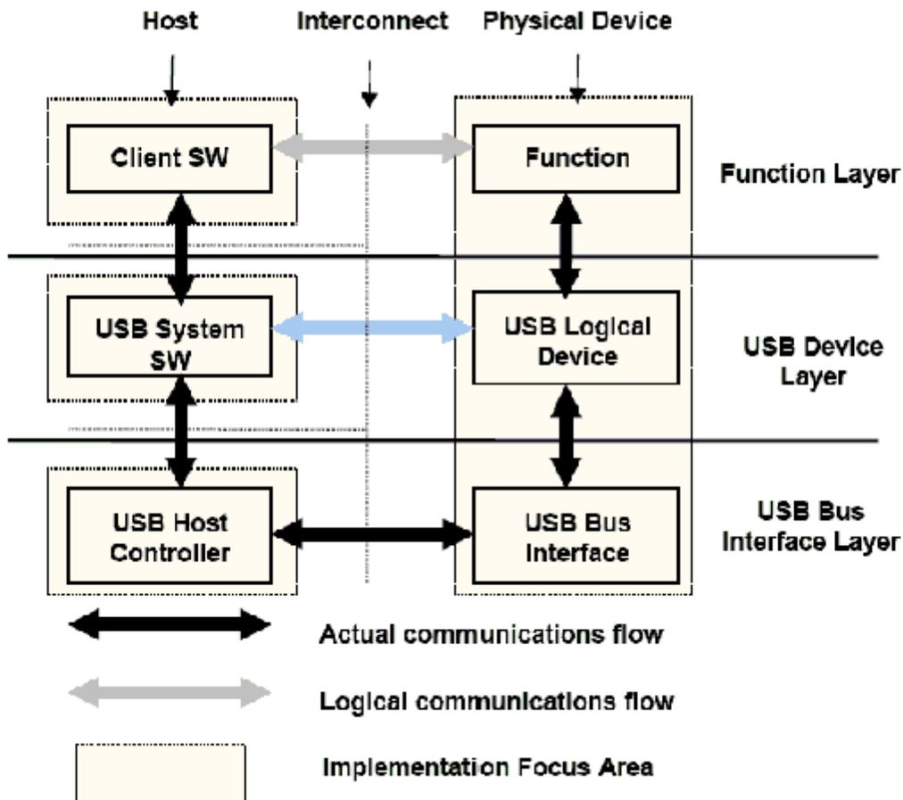
Figure 35-1. USB Block Diagram
