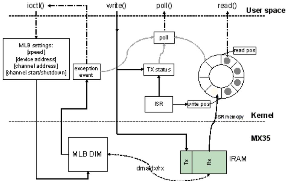
**Figure 34-2. MLB Driver Architecture Diagram**
