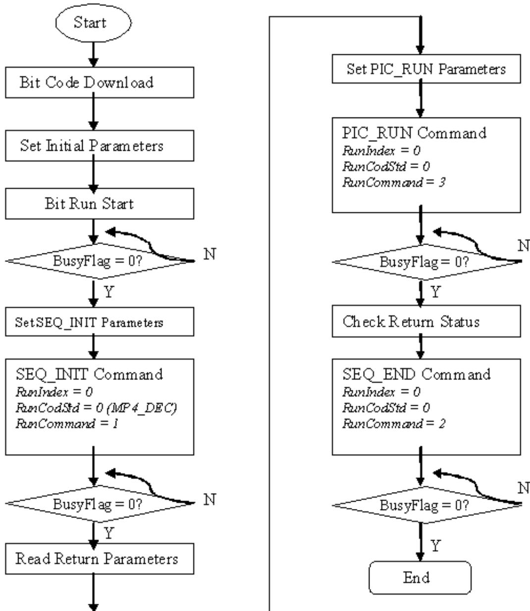
Figure 15-1. VPU Hardware Data Flow
