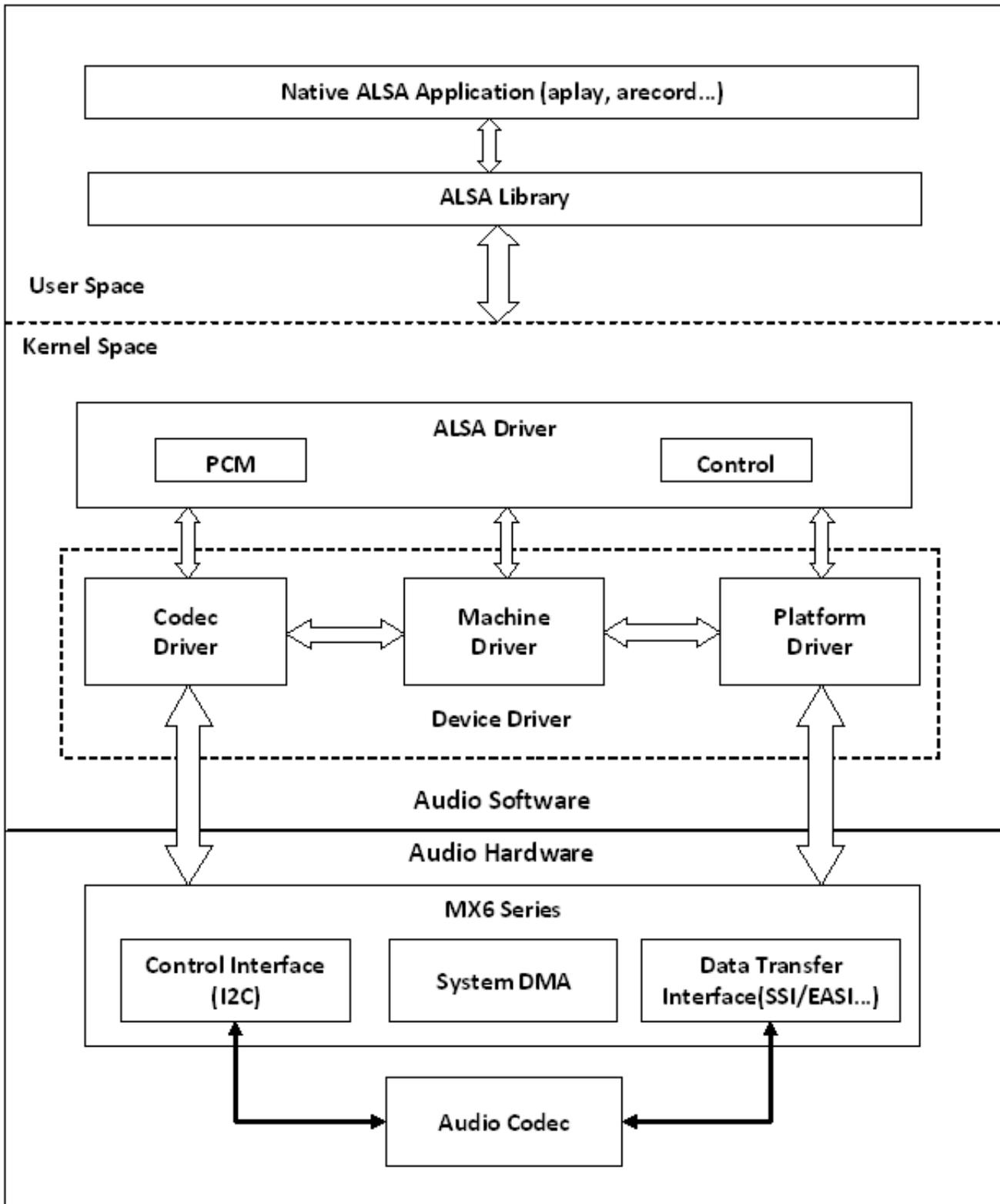
Figure 25-1. ALSA SoC Software Architecture
