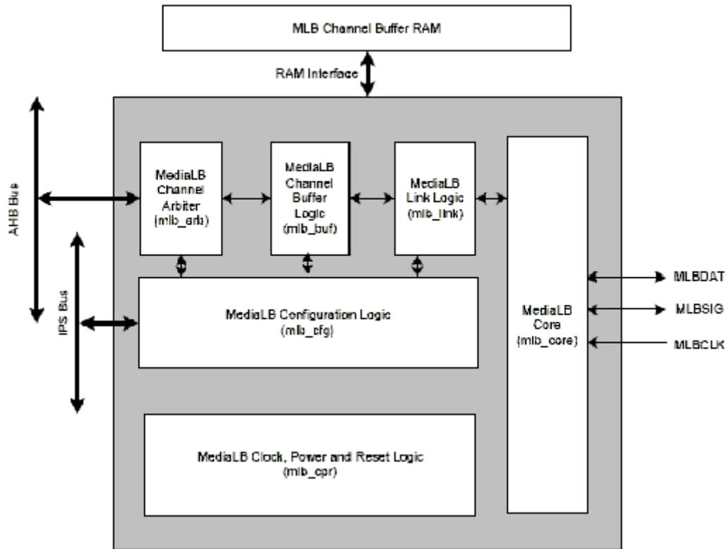
**Figure 34-1. MLB Device Top-Level Block Diagram**
