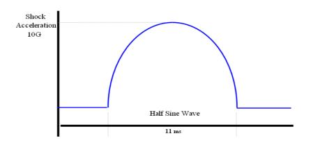
System condition : operation (running burn in test program )
