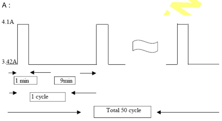
The adapter shall support a surge load with 120% of maximum load for 1min , maximum load for 9min and Output Voltage more than 18.05V at input voltage is 100-240Vac
